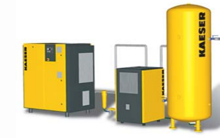
Variant 2 For heavily fluctuating air demand, the SECOTEC® dryer is located between the compressor, centrifugal separator and air receiver.
