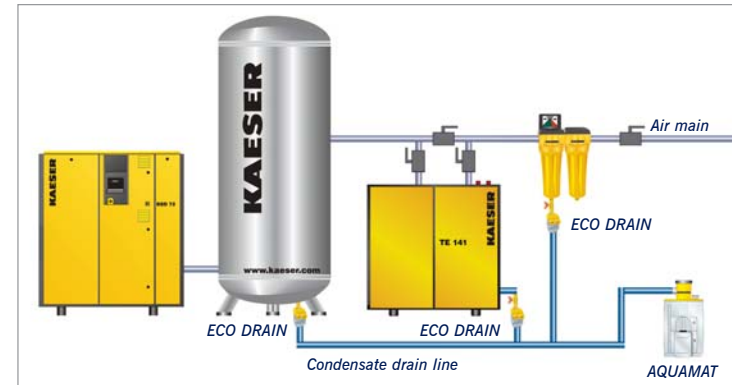
All collection points must be fitted with a reliable means of draining condensate. Best results are achieved with an electronically controlled condensate drain.
