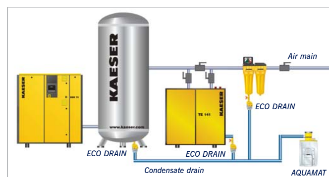
All collection points must be fitted with a reliable means of draining condensate. Best results are achieved with an electronically controlled condensate drain.
