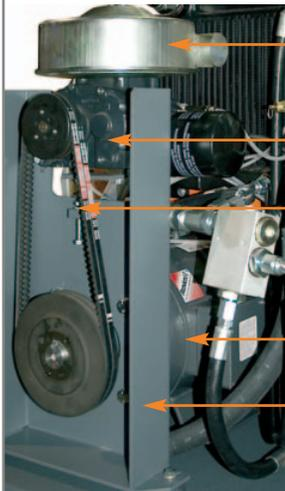
LARGE AREA 3 MICRON AIR INTAKE FILTER
