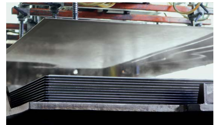
Compressed air from the Kaeser station plays a vital role in the largely automated production process for Eternit facade panels
