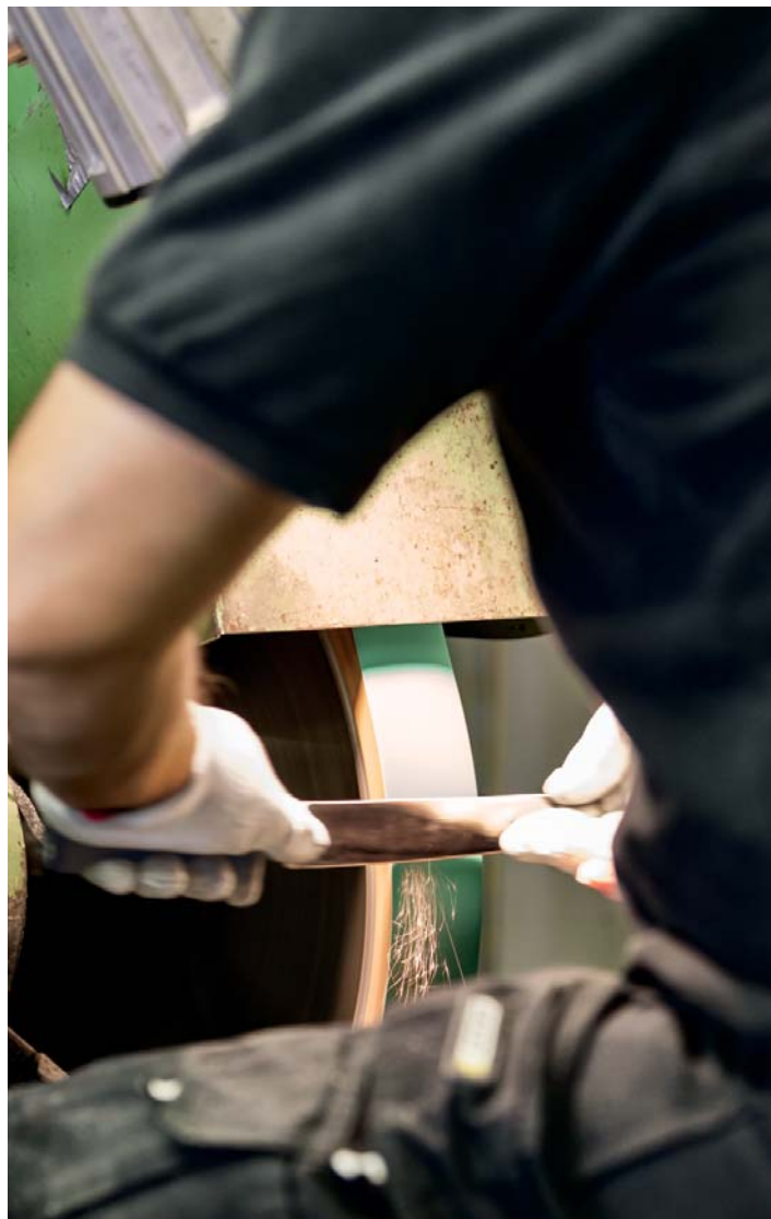
Following final finishing, the blades are razor sharp
