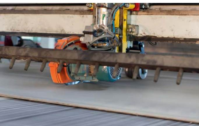
Compressed air is even used in the cutting process for the facade panels
