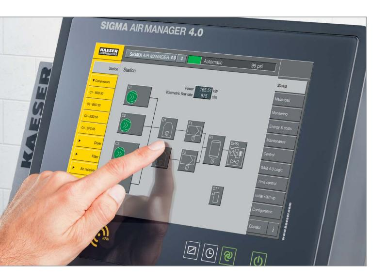
Kaeser's Sigma Air Manager 4.0 (SAM) can control up to 16 blowers and only turns them on when needed to meet air demand. This improves system stability, reduces energy use, and equalizes blower run time.
