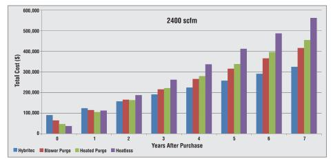
For 2400 cfm, Hybritec's total costs, including purchase are lower than other types of dessicant dryers after only 2 years. For 5300 cfm, Hybritec breaks even with other dryers in less than a year. Based on 8760 hours of operation at \$0.10/kWh running desiccant dryer 7 months.
