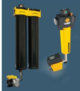
All desiccant dryers require proper filtration. Coalescing pre-filters prevent contamination of desiccant beds by hydrophobic aerosols. Particulate after-filters collect traces of desiccant dust that may exit the dryer. Maintaining these filters extends service intervals and provides excellent air quality. All Kaeser desiccant dryers offer optional filter packages with or without block and bypass valves.
