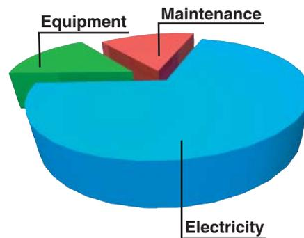
Analyze the total cost of a compressed air system and you'll realize that power cost is significant. In just one year it could exceed the cost of the compressor itself. Over a period of ten years, this could consume 70% of your overall costs.
