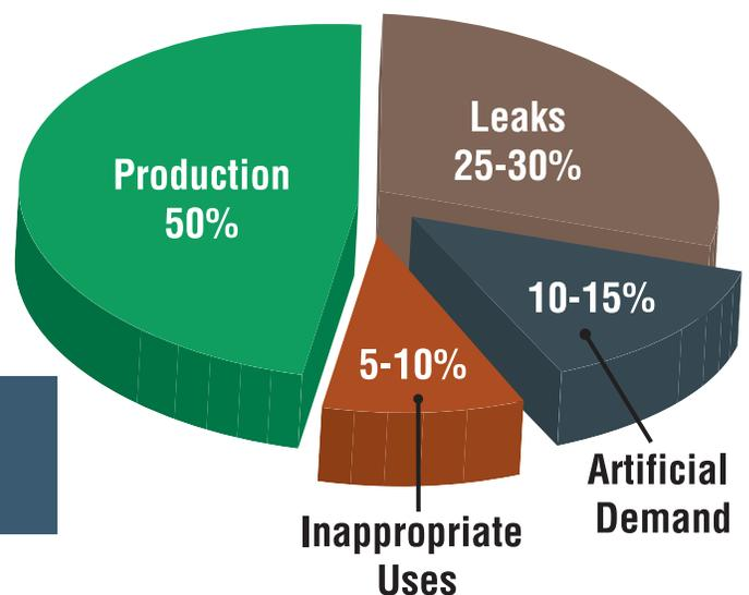
*The U.S. Department of Energy estimates that only 50% of compressed air is put to productive use – meaning most air systems have significant energy saving potential.*
