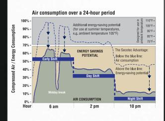
The graph shows a typical compressed air consumption profile. Secotec dryers save energy because the refrigerant system is shut down during breaks, periods of low demand, and downtime; the control system operates without fixed run-on periods. The integrated thermal mass ensures that the system is always ready for operation.
