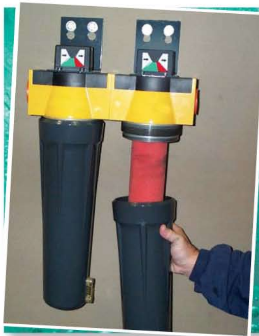
Make sure changing your air compressor's filters is on your maintenance schedule.
